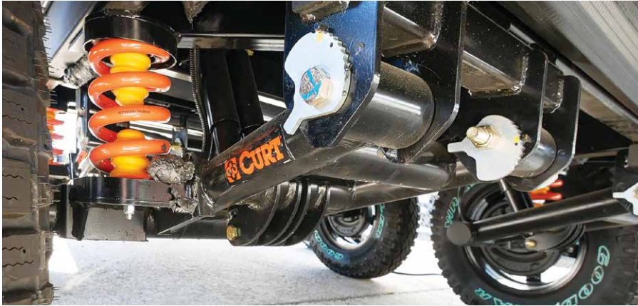
CURT BEAST MODE INDEPENDENT SUSPENSION SYSTEM WITH GOODYEAR ALL-TERRAIN TIRES
