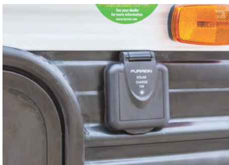
Solar Prep and Wiring
